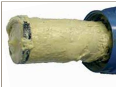
Close up of the 'mayonnaise' removed from a compressed air supply, prior to entering a desiccant air dryer. The dryer's operating life was improved as it now removes water vapour
