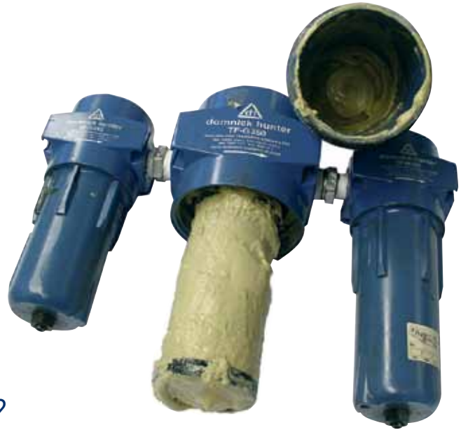
Contamination removed by a Parker domnick hunter water separator and high-efficiency coalescing filters fitted before a desiccant air dryer
