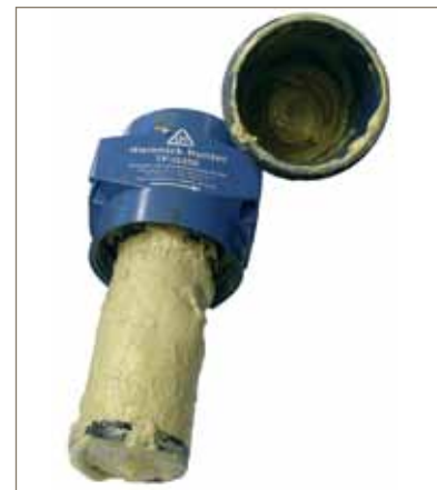
Typical contamination removed by a Parker domnick hunter locomotive filter
